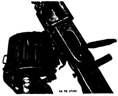
Figure 22 — Mounting Belt Drum Magazine 23
