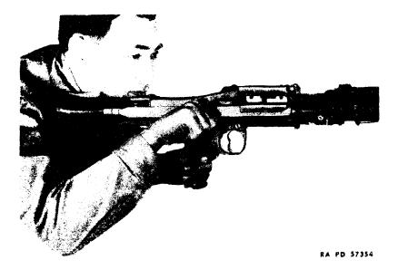
Figure 30 - Cocking Handle in Forward Position - Gun Cocked
