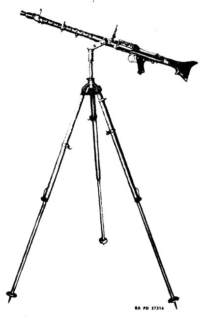
Figure 4 — Machine Gun — on Antiaircraft Tripod
