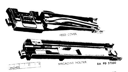
figure 24 - Feed Cover and Magazine Holder - Bottom View
