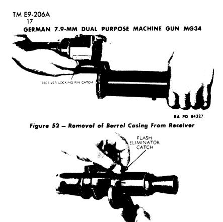
Figure 53 - Removal of Blast Trap and Flash Eliminator
