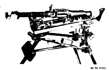
Figure 10 — Mounting the Machine Gun on the Tripod Mount
