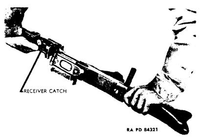
Figure 39 — Unlocking and Rotating Receiver
