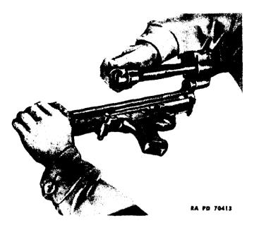
Figure 51 – Removal of Barrel 45
