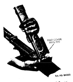
Figure 25 – Removal of Feed Cover
