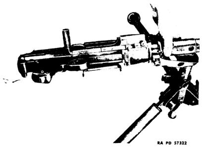
Figure 8 - Mounting Machine Gun on Antiaircraft Tripod
