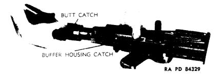
Figure 46 — German 7.9-mm Dual Purpose Machine Gun MG34 — Removal of Butt
