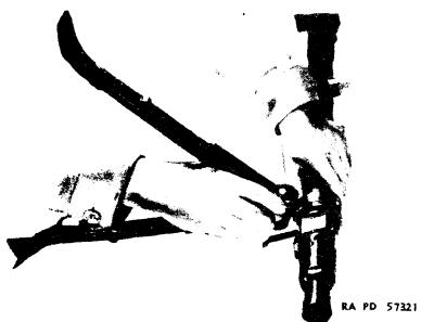
Figure 6 - Mounting Machine Gun on Bipod
