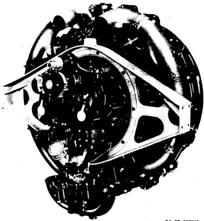
Figure 2 - R975-C1 Engine - Right Rear View
