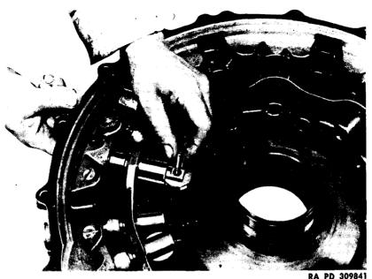
Figure 96 – Installing Tappet Roller Pins and Rollers
