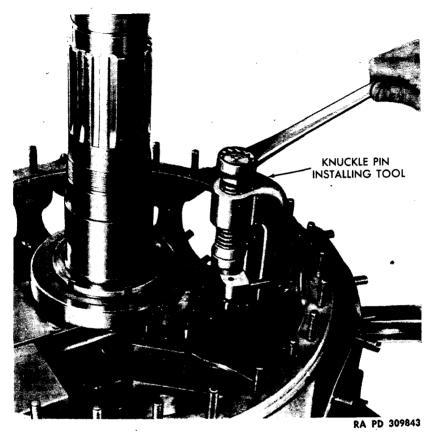
Figure 98 - Installing Connecting Rod Knuckle Pins
