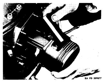
Figure 140 – Installing Piston Pin
