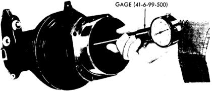
Figure 75 - Checking Cylinder Bore for Wear RA PD 336200
