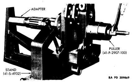
Figure 69 - Removing Plug From Rear Crankshaft
