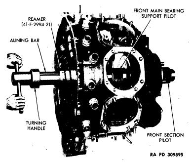
Figure 89 — Reaming Crankshaft Rear Main Bearing
