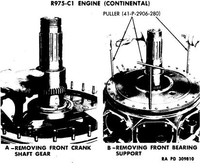
Figure 44 — Removing Front Main Bearing Support and Crankshaft Gear
