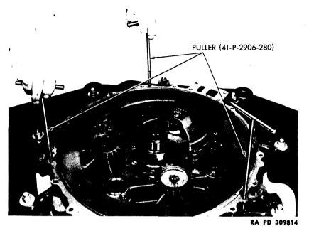
Figure 51 – Removing Crankcase Diffuser Section From Rear Section
