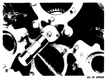
Figure 126 – Installing Generator Idler Gear Shaft
