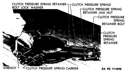
Figure 168 - Removing Clutch Pressure Spring Retainers
