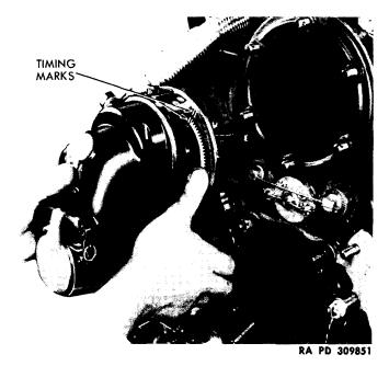
Figure 150 – Installing Magneto (Scintilla)
