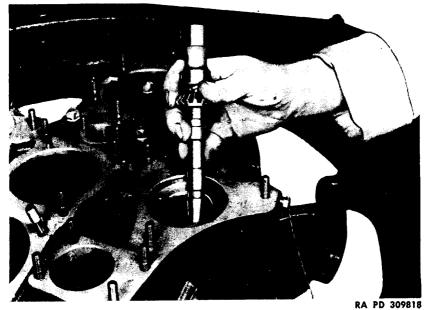
Figure 121 – Removing Accessory Drive Shaft Assembly (Magneto Drive)
