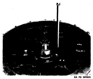
Figure 107 — Removing Impeller Drive Shaft Support Screws
