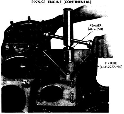
RA PD 309906 Figure 123 — Line Reaming Accessory Drive Shaft Bushing
