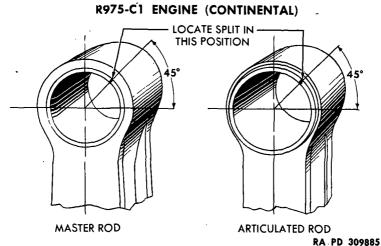
Figure 83 - Connecting Rods, Showing Location of Split in Bushing
