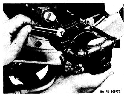
Figure 12 – Removing Governor Flange Nuts
