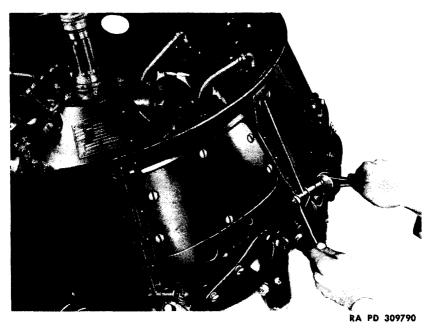
Figure 21 – Removing Nut and Bolt From Cowl Attaching Boss
