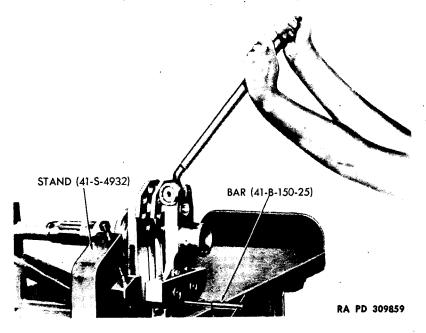
Figure 95 - Tightening Rear Crankcheek Cap Screw
