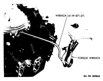
Figure 142 - Tightening Cylinder Hold-down Nuts
