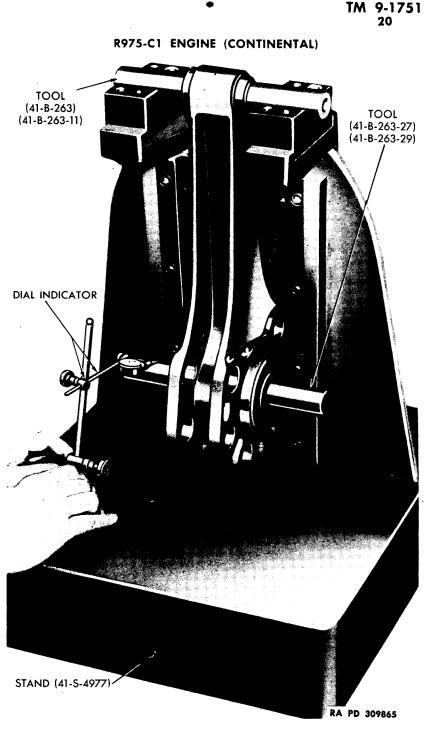
Figure 78 - Checking Master Rod Alinement
