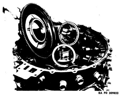
Figure 62 -- Removing Cam, Spacer, and Bearing
