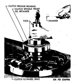
Figure 174 – Installing Spindle Front Bearing Oil Retainer, Using Drift (41-D-1540-800)
