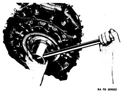
Figure 60 – Removing Cam Hub Bearing Support
