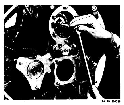
Figure 46 - Removing Cranking Motor Shaft Nut
