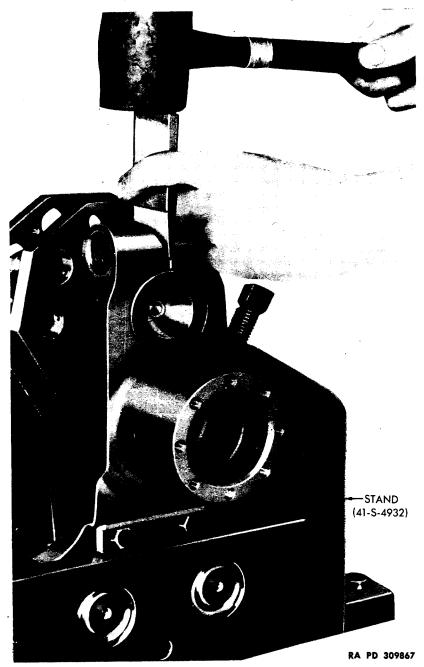
Figure 66 - Spreading Rear Crankcheek
