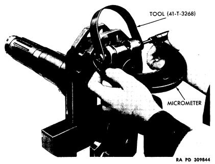
Figure 94 - Measuring Crankcheek Cap Screw Stretch
