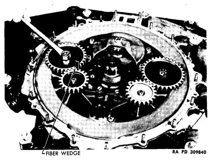
Figure 136 – Tightening Accessory Drive' Gear Nut
