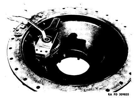
Figure 53 - Removing Front Section Scavenge Pump Gear Nut
