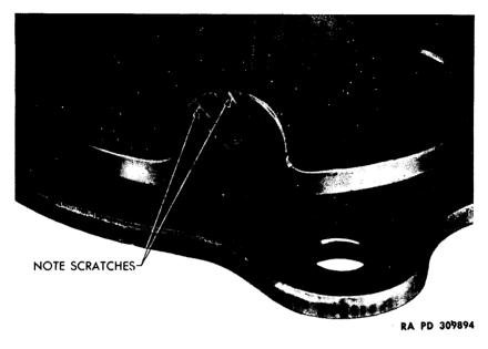
Figure 122 - Generator Drive Gear Support
