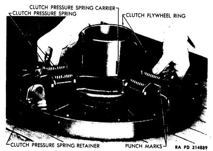
Figure 167 - Removing Pressure Spring Carrier
