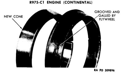
Figure 56 - Flywheel Hub Rear Cone
