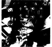
LOOSENING ROMEC PUMP FLANGE NUTS
