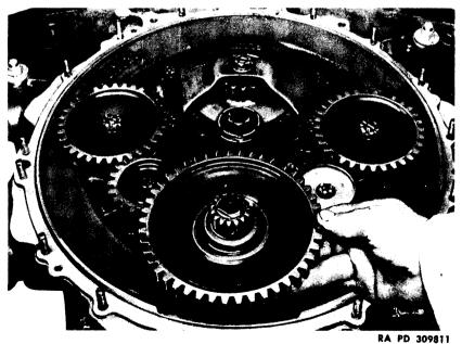
Figure 48 – Removing Cranking Motor Drive Gear and Cam Drive Pinion
