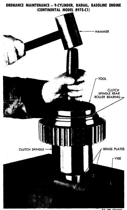
RA PD 336907 Figure 175 – Installing Spindle Rear Bearing, Using Drift (41-D-1540-150)
