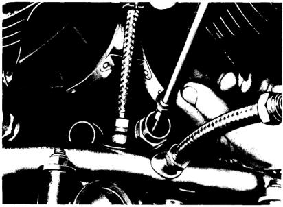
Figure 30 - Removing Valve Tappet Ball Socket and Spring
