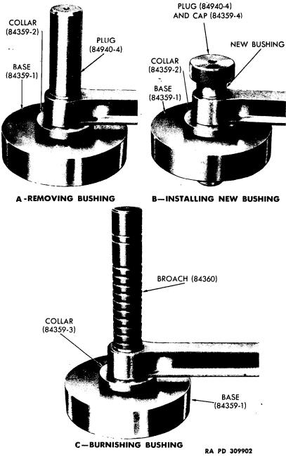
Figure 82 — Replacing Piston Pin Bushing in Articulated Rod
