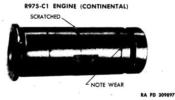
Figure 76 – Articulated Rod Knuckle Pin
