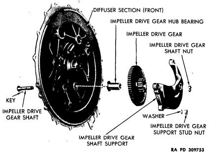
Figure 113 - Impeller Drive Gear, Shaft, and Support Disassembled
