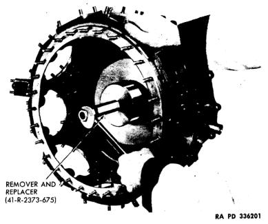
Figure 87 - Removing Rear Main Bearing
