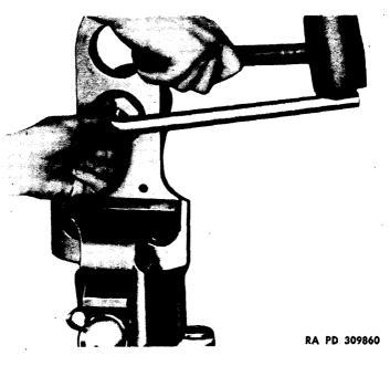
Figure 91 – Tightening Rear Crankshaft Front Plug
