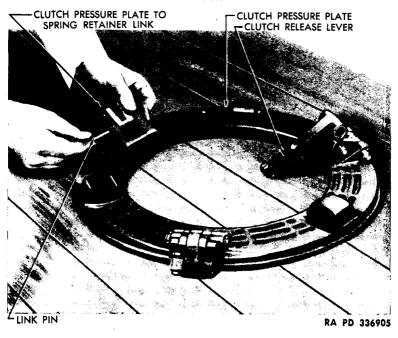
Figure 169 – Removing Pressure Plate to Release Lever Link
