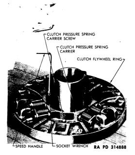
Figure 166 - Removing Pressure Spring Carrier Cap Screws
