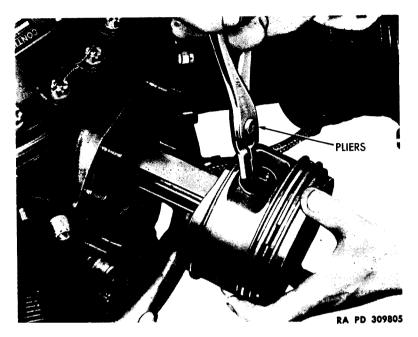
Figure 38 - Removing Piston Pin Retainer
