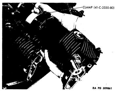
Figure 141 – Installing Cylinder
