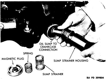
Figure 39 – Removing Oil Sump Strainer Assembly
