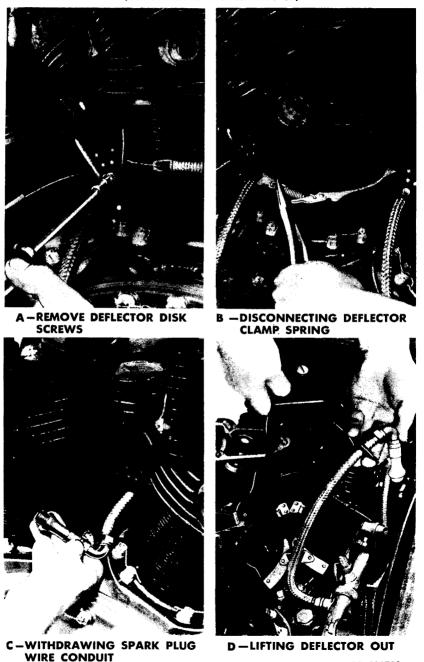
Figure 32 – Removing Intercylinder Air Deflector
