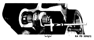
Figure 133 - Oil Pressure Relief Valve Setting
