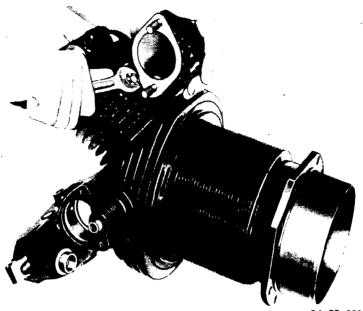
RA PD 309826 Figure 71 — Removing Exhaust Elbow, Using Wrench (41-W-1471)
