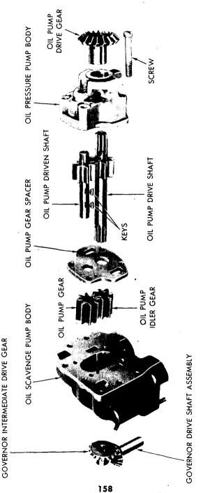
Figure 130 - Main Oil Pump Disassembled
