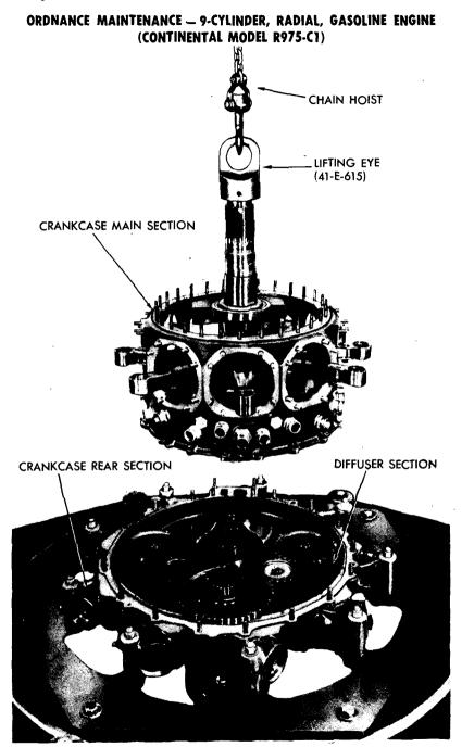
RA PD 309762 Figure 45 — Raising Crankcase Main Section From Diffuser and Rear Sections
