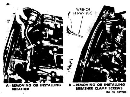
Figure 25 – Removing Atmospheric Breather
