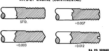
Figure 52 — Identification of Oversize Studs
