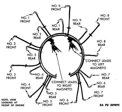
Figure 101 – Ignition Wiring Harness
