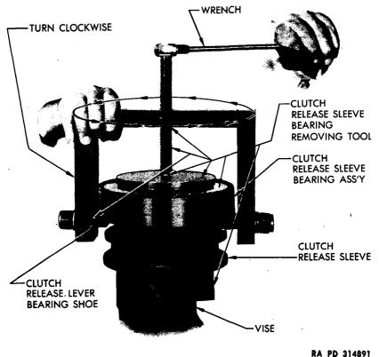
Figure 170 – Removing Clutch Release Sleeve Bearing, Using Puller (41-P-2906-75)
