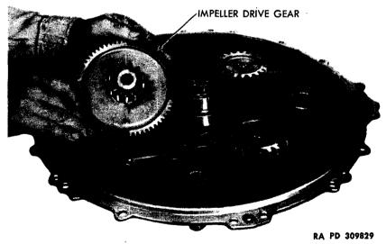
Figure 104 - Removing Impeller Drive Gear
