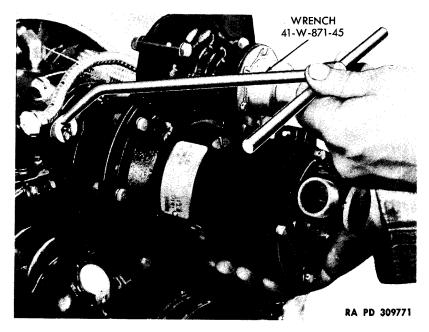
Figure 10 – Removing Cranking Motor Flange Nuts
