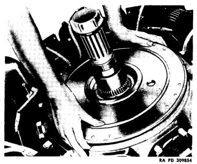
Figure 138 — Installing Front Main Bearing Support
