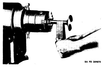
Figure 72 - Polishing Valve Stem
