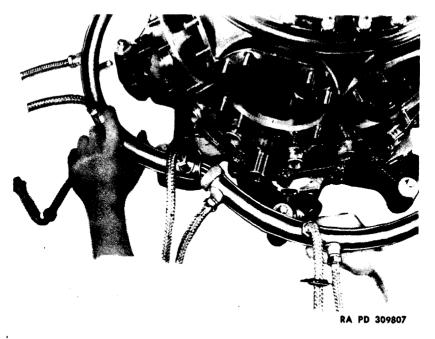
Figure 41 - Lifting Off Ignition Harness
