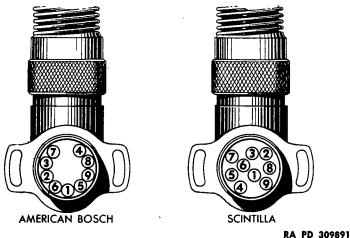
Figure 102 - Position of Wires Through Cable Outlet Adapter
