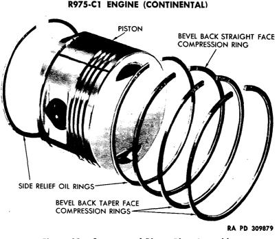
Figure 99 - Sequency of Piston Ring Assembly
