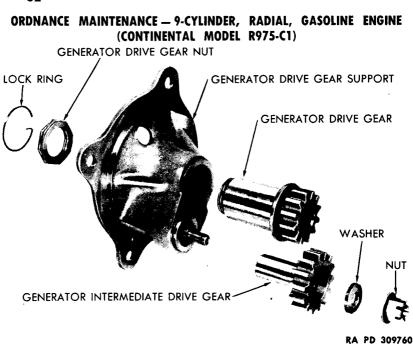
Figure 127 – Generator Drive Gear and Support Assembly Disassembled
