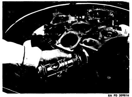
Figure 119 – Removing Tachometer and Three-way Accessory Drive Adapter
