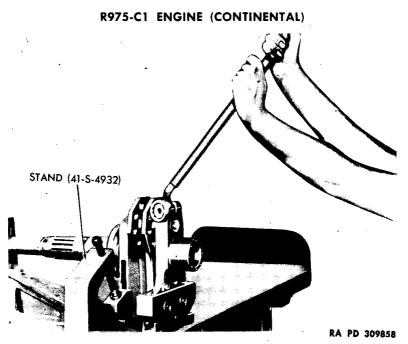
Figure 65 - Loosening Rear Crankcheek Cap Screw
