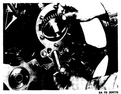
Figure 118 - Removing Generator Idler Gear
