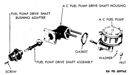
Figure 128 — A-C Fuel Pump and Adapter Assembly Disassembled THREE-WAY ACCESSORY DRIVE GEAR
