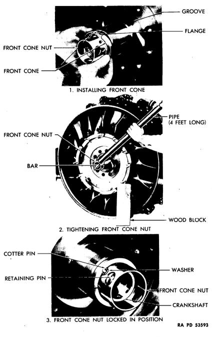
Figure 153 – Installing Front Cone and Nut
