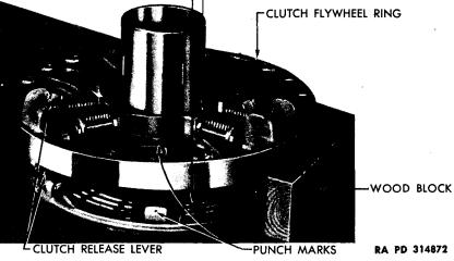
Figure 164 - Pressure Plate Removed From Flywheel Ring
