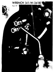
A -LOOSEN OR TIGHTEN TACHOMETER DRIVE NUTS
