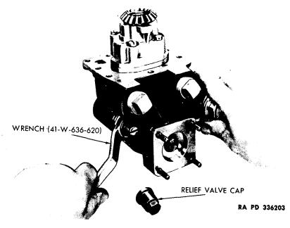
Figure 115 - Removing Oil Pressure Relief Valve
