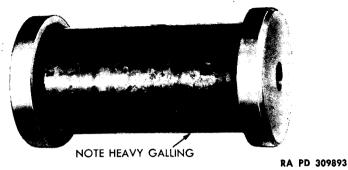
Figure 79 - Rear Counterweight Pin
