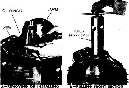
COVER SHIM AND OIL SLINGER Figure 43 – Removing Crankcase Front Section Cover, Shim, Oil Slinger, and Housing
