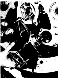
A-LOOSENING OR TIGHTENING THREE-WAY ACCESSORY DRIVE HOUSING NUTS
