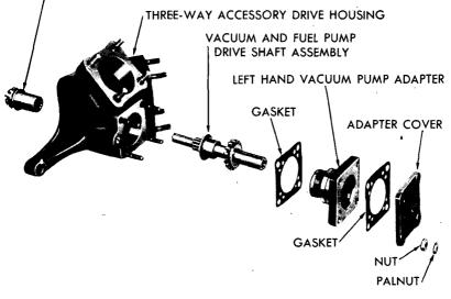
RA PD 309754 Figure 129 — Three-way Accessory Drive Housing and Fuel Pump Drive Shaft Disassembled
