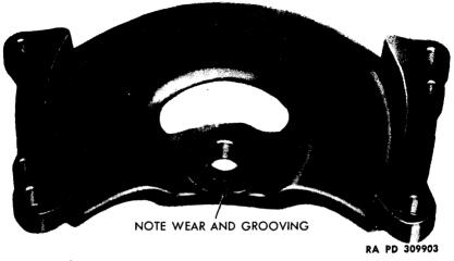
Figure 109 — Impeller Drive Gear Shaft Support
