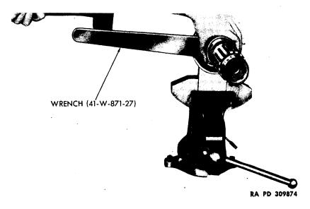
Figure 67 - Loosening Front Main Bearing Lock Nut
