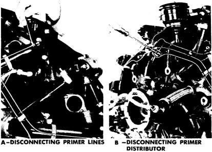
Figure 22 - Removing Priming System
