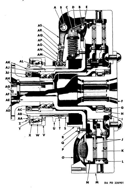
Figure 159 - Clutch Assembly - Sectional View
