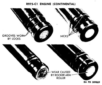
Figure 73 - Valve Stems, Worn and Damaged in Service
