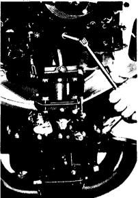
B -REMOVE CARBURETOR FLANGE NUTS
