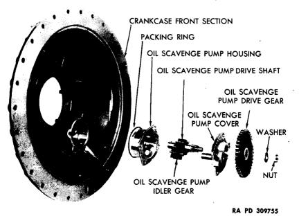
Figure 57 — Front Section Scavenge Oil Pump Disassembled
