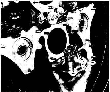
RA PD 309780 Figure 116 — Removing Generator Drive Gear Assembly
