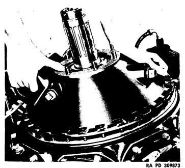
Figure 139 — Installing Crankcase Front Section
