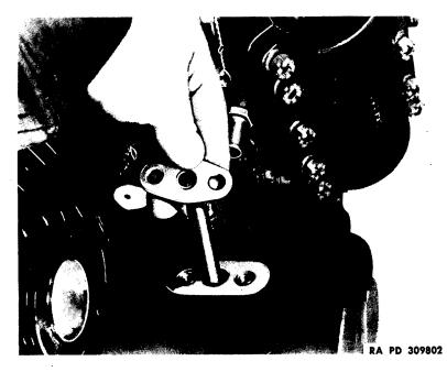
Figure 35 — Removing Oil Sump Internal Tube
