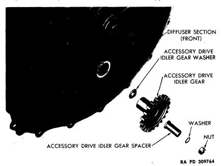
Figure 114 - Accessory Drive Idler Gear
