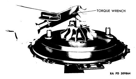
Figure 112 - Tightening Impeller Rear Nut
