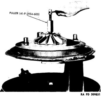
Figure 106 – Removing Supercharger Impeller
