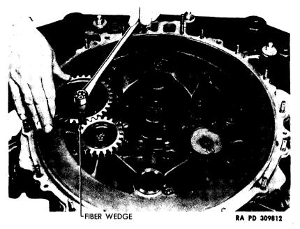
Figure 49 - Removing Accessory Drive Gear Nut (Magneto Drive)
