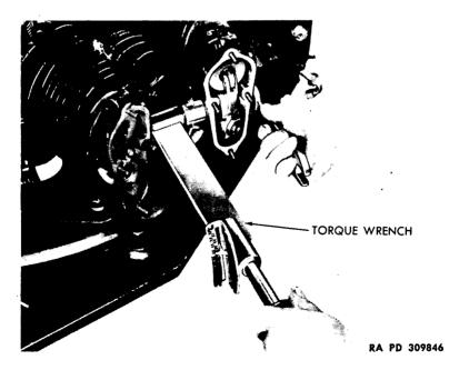
Figure 144 – Tightening Rocker Arm Hub Bolt and Nut
