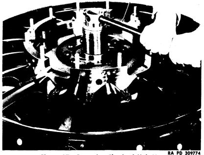
Figure 17 – Removing Flywheel Hub Nut
