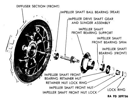
Figure 110 — Impeller Drive Shaft Gear and Support Disassembled
