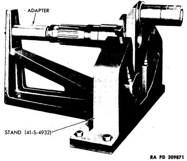
Figure 64 - Crankshaft Disassembly and Assembly Stand
