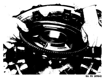
Figure 97 – Installing Cam and Bearing Assembly
