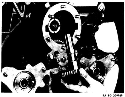
Figure 47 – Removing Cranking Motor Shaft
