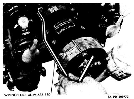
Figure 11 – Removing Generator Flange Nuts
